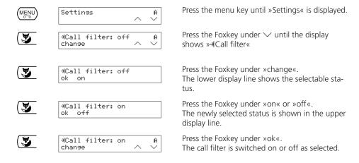
☐ If the call filter is active, the status pictogram ¾ indicates this in the standby display.
