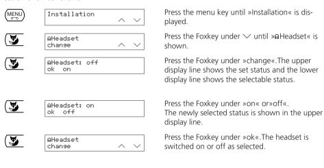
$\Box$  If the headset is switched on, the status pictogram  $\Box$  indicates this in the standby display.
