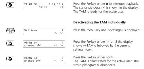
You can also activate and deactivate the TAM using speed-dialling (for the active user) (see »Speed-dialling«).
